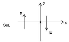
Force due to Electric field is along -y axis and force due to  $\vec{B}$  is zero.
