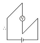
At  $t \to \infty$ , capacitor acts as open circuit & no current flows through voltmeter.
