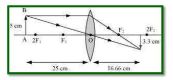
The negative value of image height indicates that the image formed is inverted. The position, size, and nature of image are shown in the following ray diagram.
